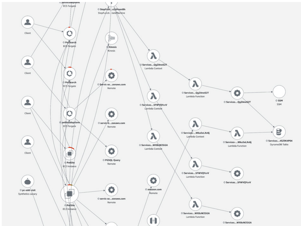
Figure 4.4 – Partial service map of a microservice architecture showing service interaction and potential issues on certain services
