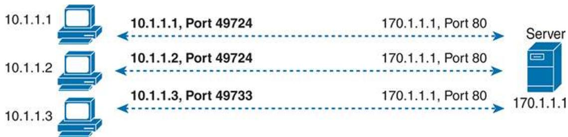
**Figure 14-6** *Three TCP Connections from Three PCs*
