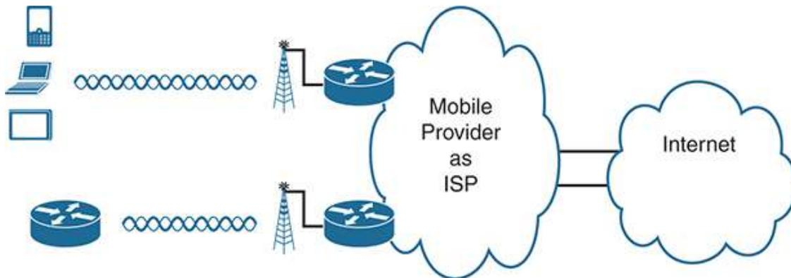
**Figure 19-16** *Wireless Internet Access Using 3G/4G/5G Technology*
