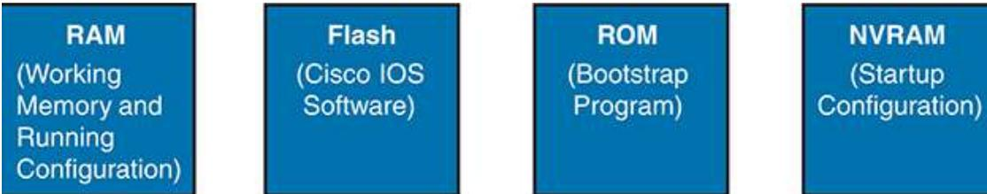
**Figure 4-13** *Cisco Switch Memory Types*
