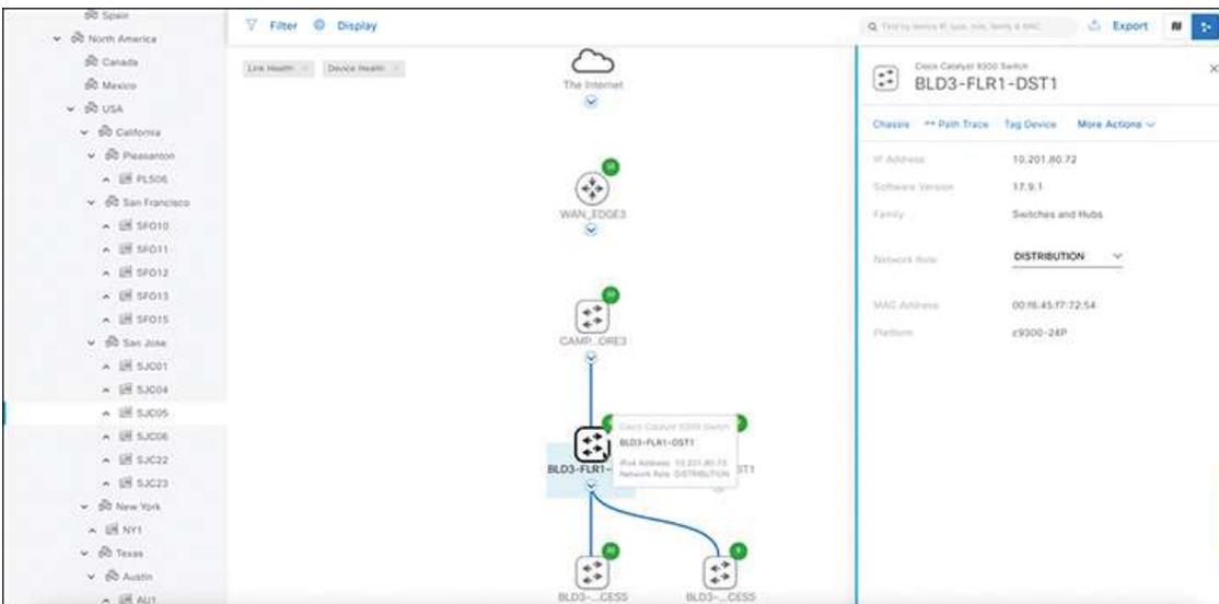
**Figure 22-17** Hover and Click Details About a Single Cisco Catalyst 9300 Switch from Cisco Catalyst Center
