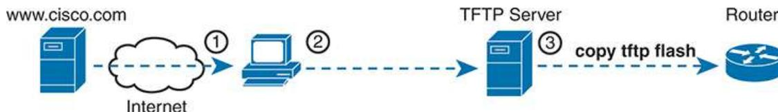
**Figure 17-7** *Copying an IOS Image as Part of the Cisco IOS Software Upgrade Process*
