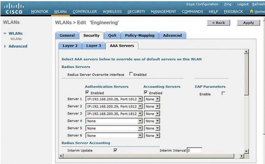
**Figure 4-33** *Selecting RADIUS Servers for WLAN Authentication*
