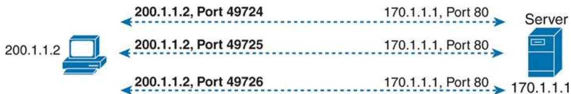
**Figure 14-7** *Three TCP Connections from One PC*
