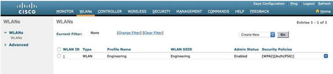
**Figure 4-36** *Displaying WLANs Configured on a Controller*
