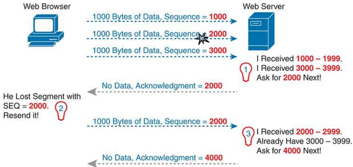
**Figure 5-8** *TCP Acknowledgment with Errors*
