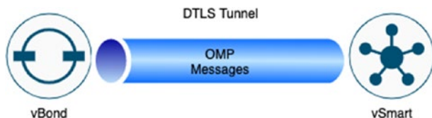
Figure 4-2. DTLS tunnel carrying OMP messages
