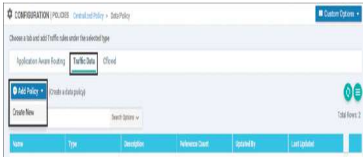
Figure 7-5 Creating a New Centralized Data Policy
