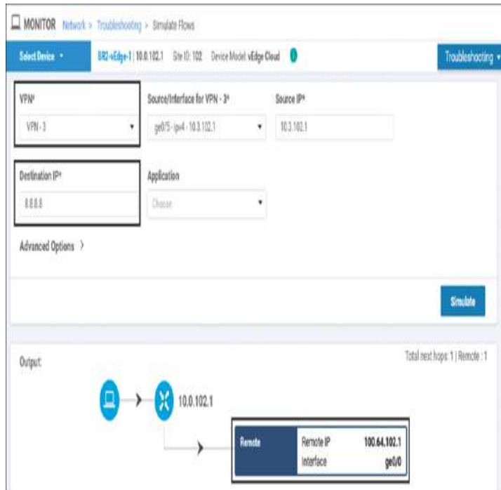
Figure 7-12 Simulate Flows Output to 8.8.8.8 from VPN 3 Shows That Traffic Is Forwarded to the Internet
