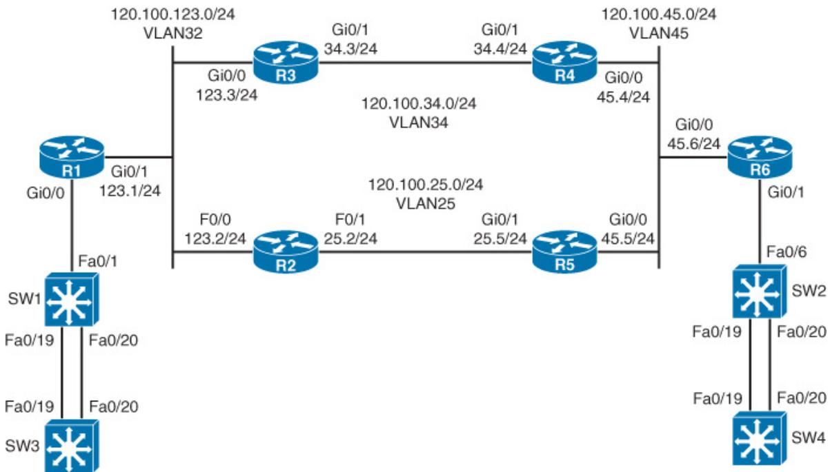
**Figure 3-3** IP Addressing Diagram
