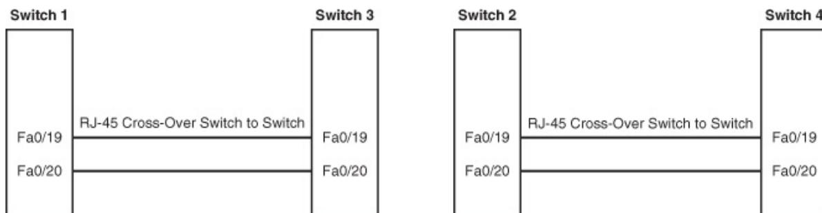
**Figure 3-2** *Switch-to-Switch Connectivity*
