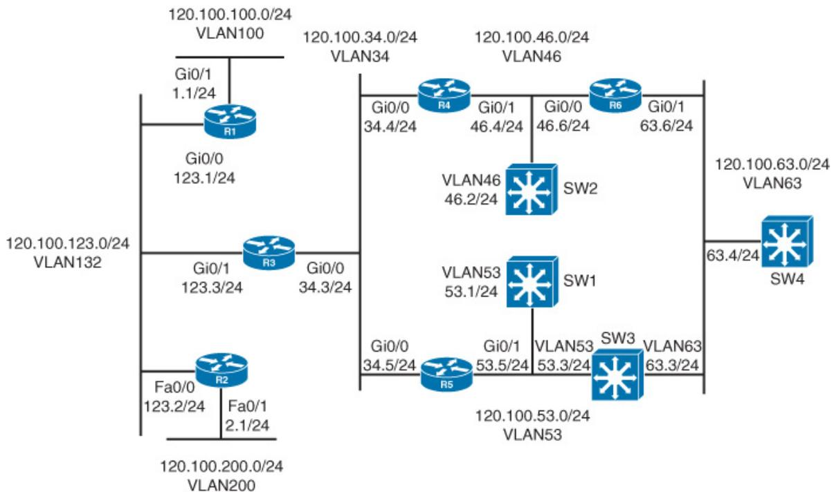
**Figure 2-4** Lab Topology Diagram
