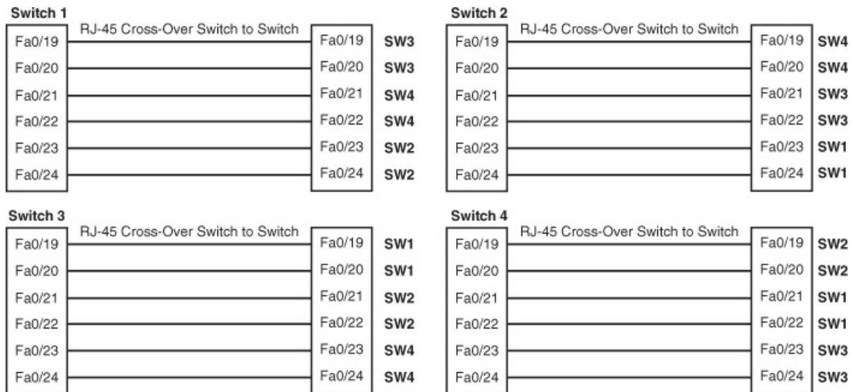
**Figure 1-2** *Switch Cabling*
