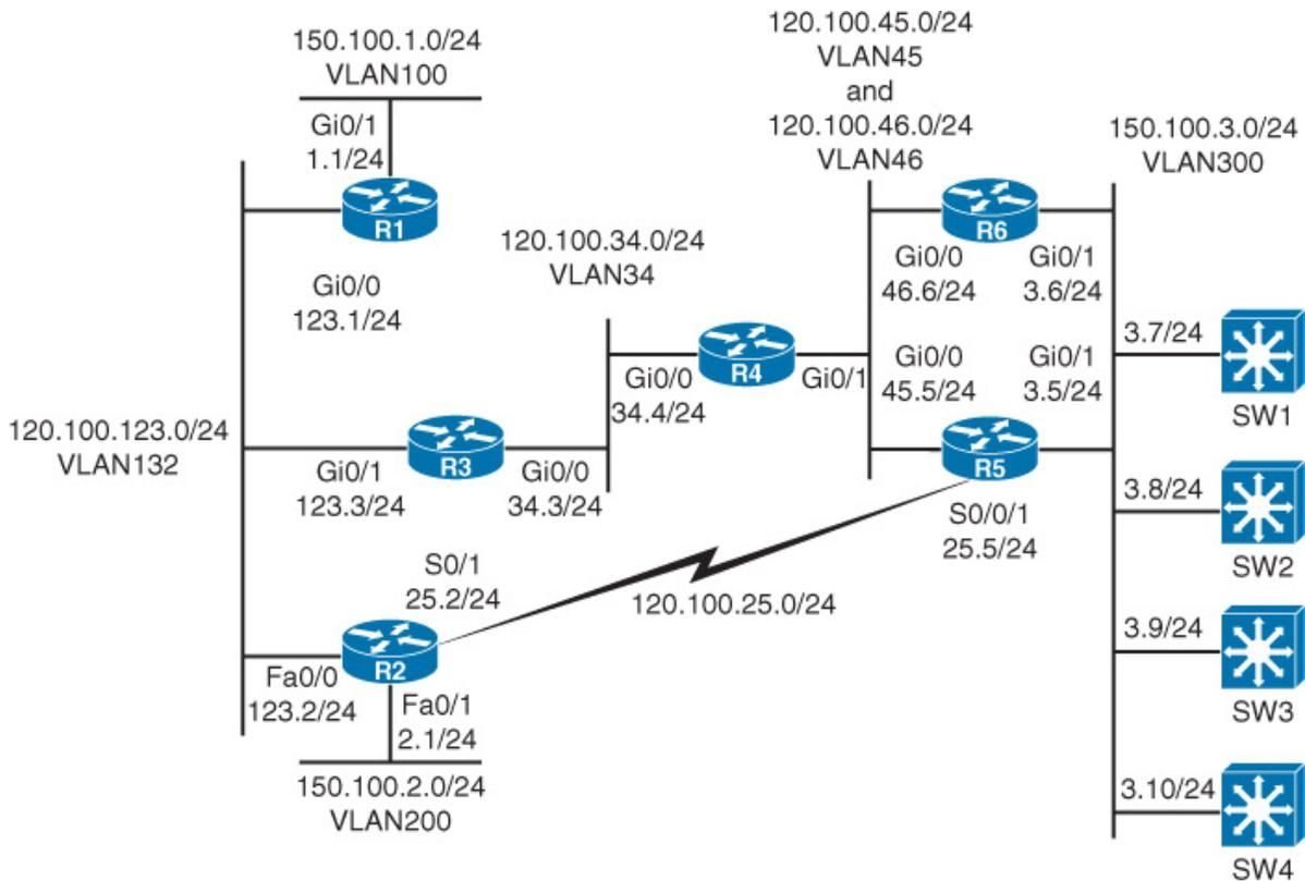
**Figure 1-3** IP Addressing Diagram
