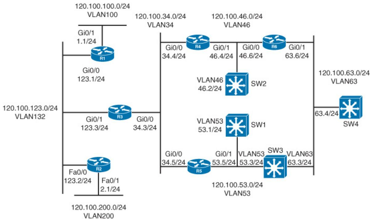
**Figure 2-3** IP Addressing Diagram
