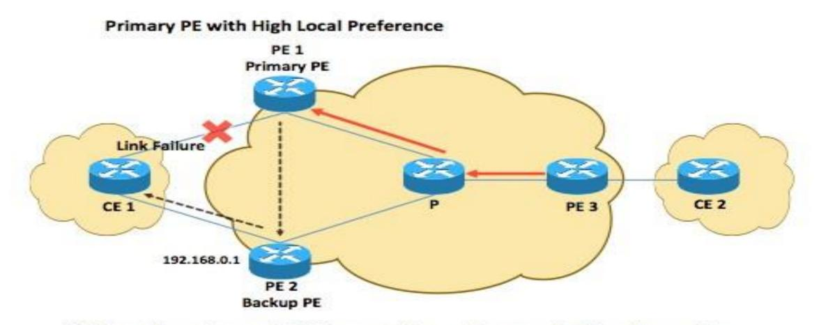
Without Best External PE3 cannot learn the standby/backup path. Best External is used for Active/Standby customer Link topologies on the Service Provider. Customer doesn't need to run BGP Best External In the above picture:
