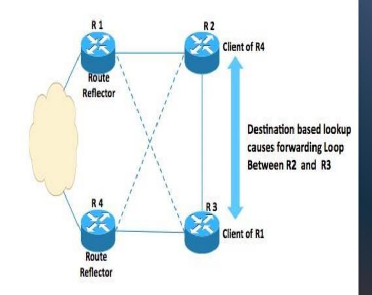
R3 should be a client of R4 instead of R1. R2 should be a client of R1 instead of R4. Then, we wouldn't have this problem  Permanent forwarding loop will occur. (Not micro-loop which is resolved automatically when the topology converged).
