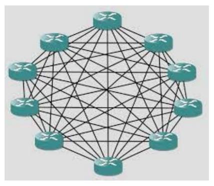
There are many design caveats when BGP RR is used, most important ones are BGP RR can create sub optimal routing, increases convergence time, reduces redundancy
