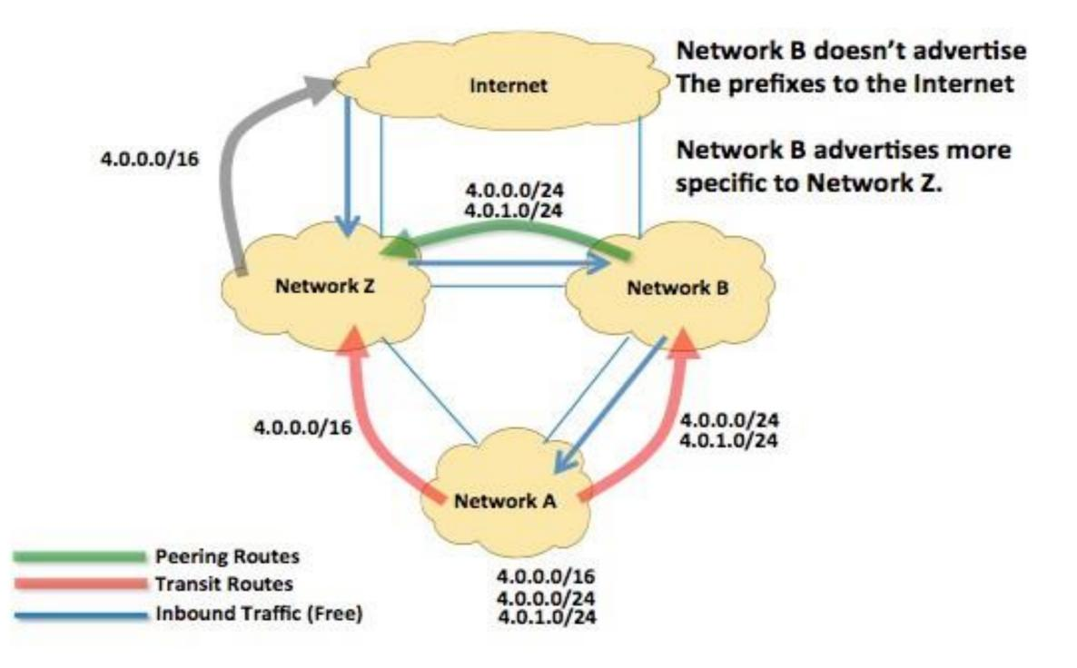
As it is depicted on the above diagram, Network B doesn't announce the specific to the world. As a result traffic from internet to Network A goes through Network Z and then through Network B over peer link
