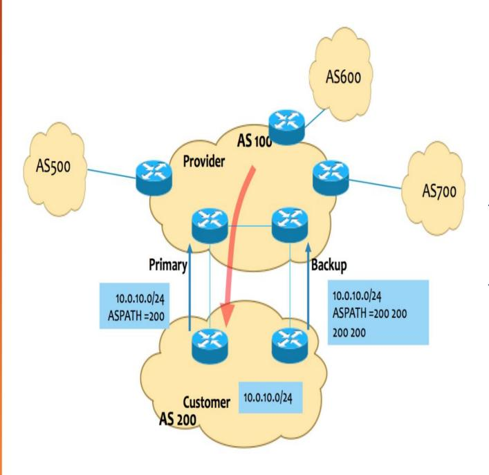
Customer AS 200 wants to use one of the links as backup. 10.0.10.0/24 prefix is sent via backup link with the 3 prepend. Thus AS path is seen through the backup link by the upstream service provider which is AS 100 as ' 200 200 200 200 '
