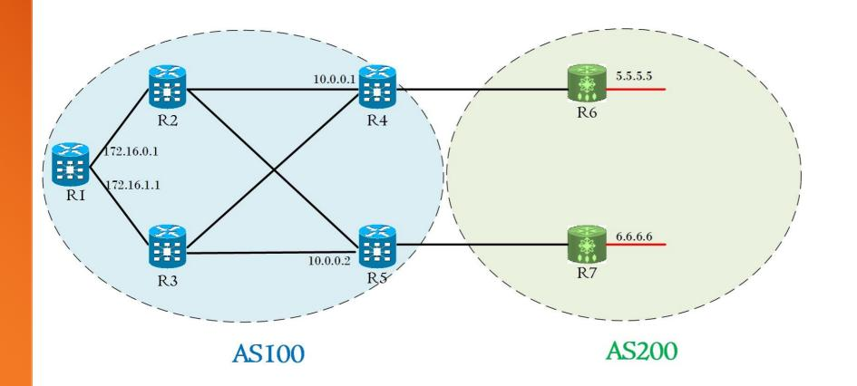
With Hierarchical FIB R1's FIB has recursive route for BGP Next hop Thus both RIB and FIB has Recursion
