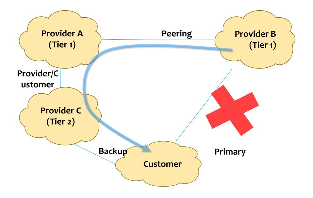
BACKUP LINK IS INSTALLED AND CAN BE USED BY THE CUSTOMER
