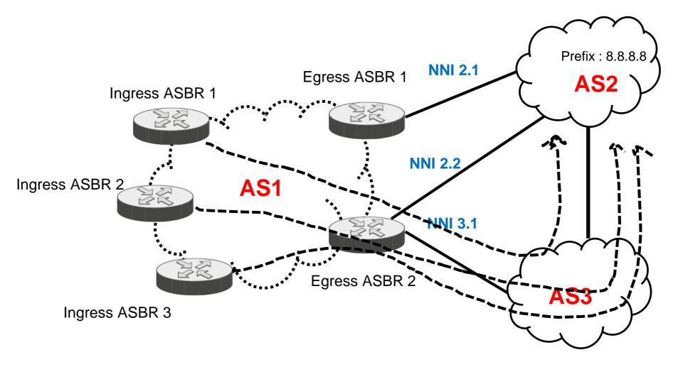
If EPE had the ability to distribute traffic among several egress links based not only on destination address, but also by considering the ingress ASBR (or ingress port etc.), this would provide much finer granularity and also bandwidth management
