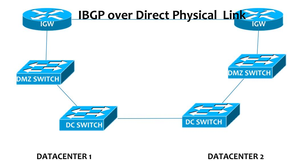
Solution 2 – Fastest option , don't require Service Provider Interaction. It should be used as a short term solution
