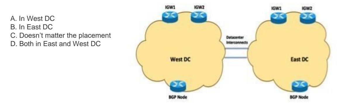
Route Reflectors should be placed in both East and West DC. Otherwise Route Reflector would choose the best path from their point of view and would send the best path to the Route Reflector Clients from their best path.
