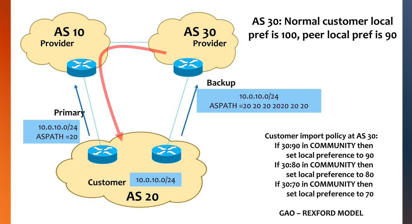
Question 5: What if customer uses second service provider link as primary and the old provider secondary and the second provider peering connection as depicted in the below topology ?
