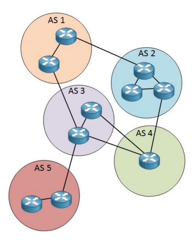
EBGP and IBGP are our main focus. If the BGP connection between two different Autonomous Systems, it is called EBGP (External BGP).
