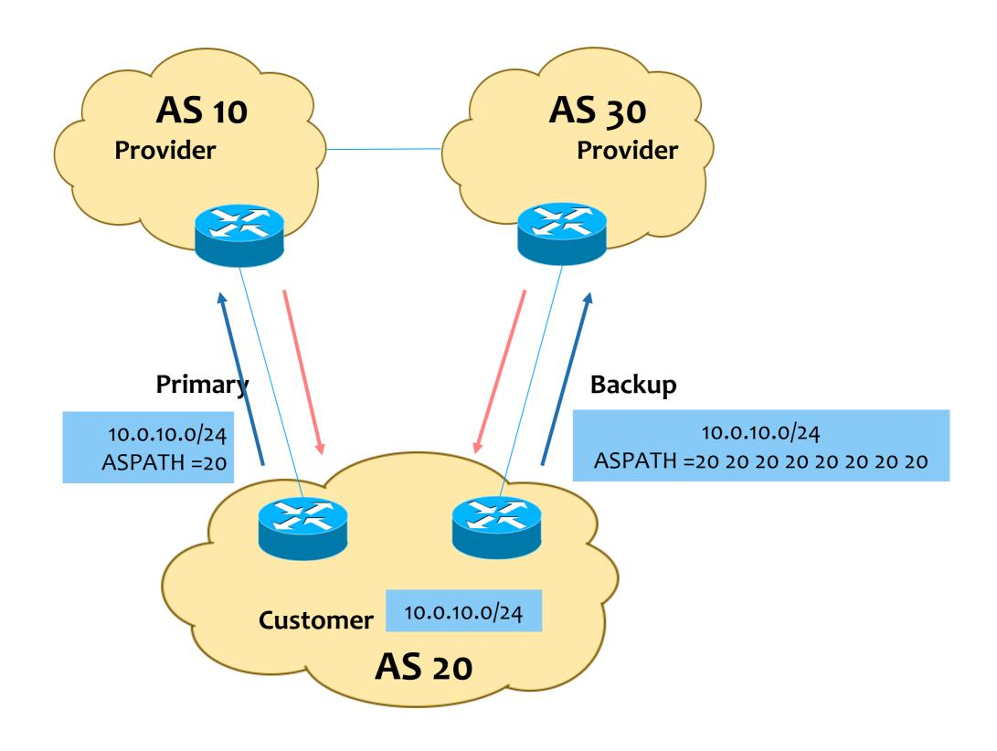
There is a problem with the design since customer wants to use second service provider as backup. AS-Path prepending in this way is often used as a form of load Balancing
