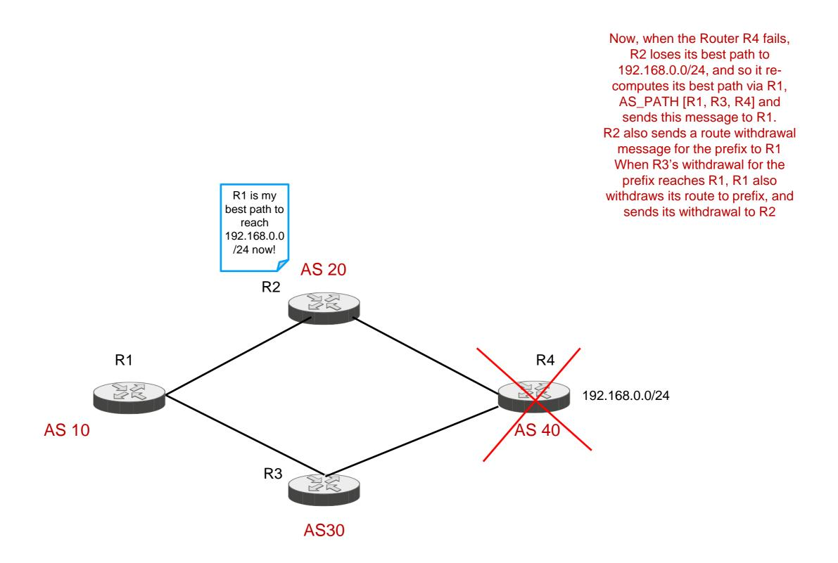
• EBGP AS number allocation will trigger path hunting when there is a failure to the destination
