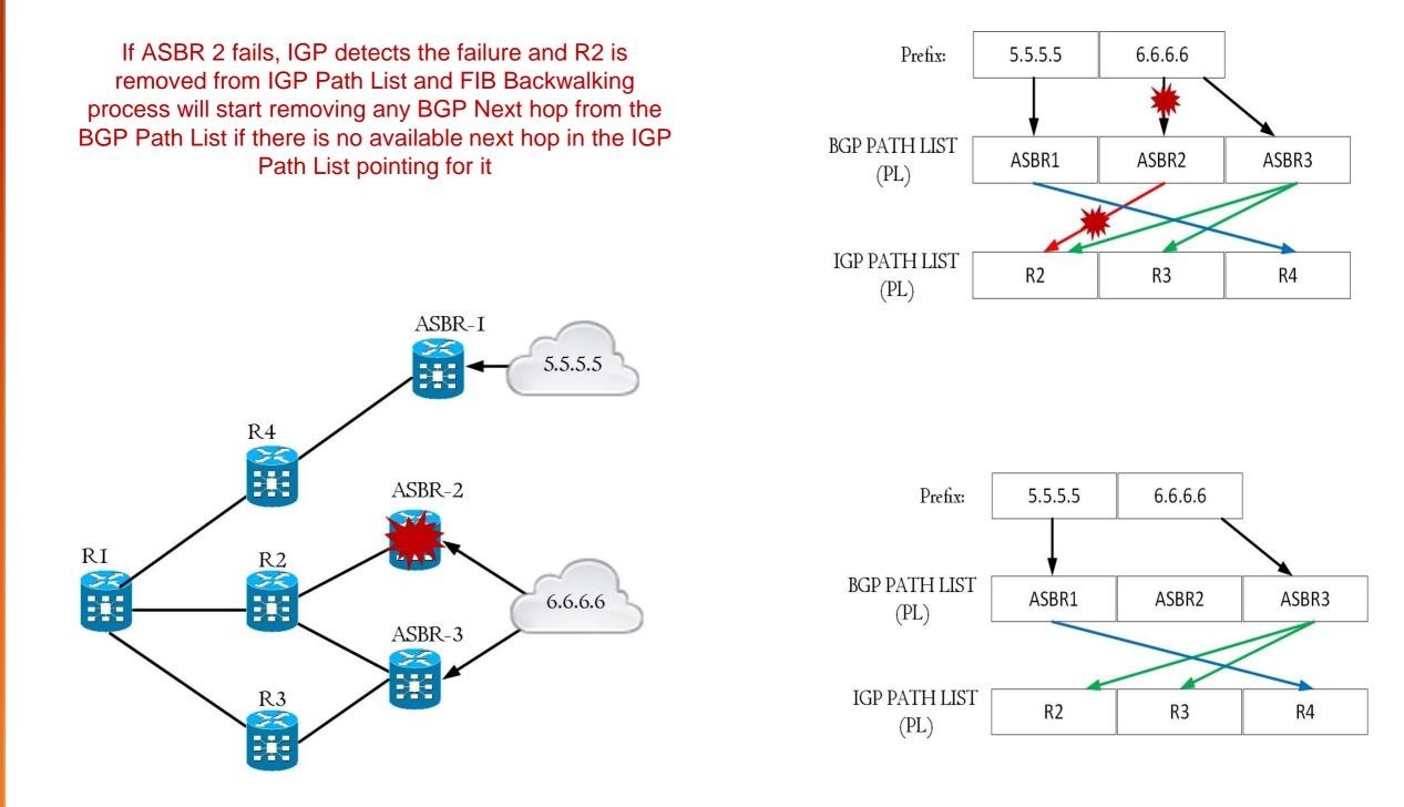
ASRB3 becomes best path immediately after ASBR 2 is removed from the BGP Path List. Backwalking process to find whether there is any BGP next hop for the external prefixes in the BGP Path List takes only couple milliseconds
