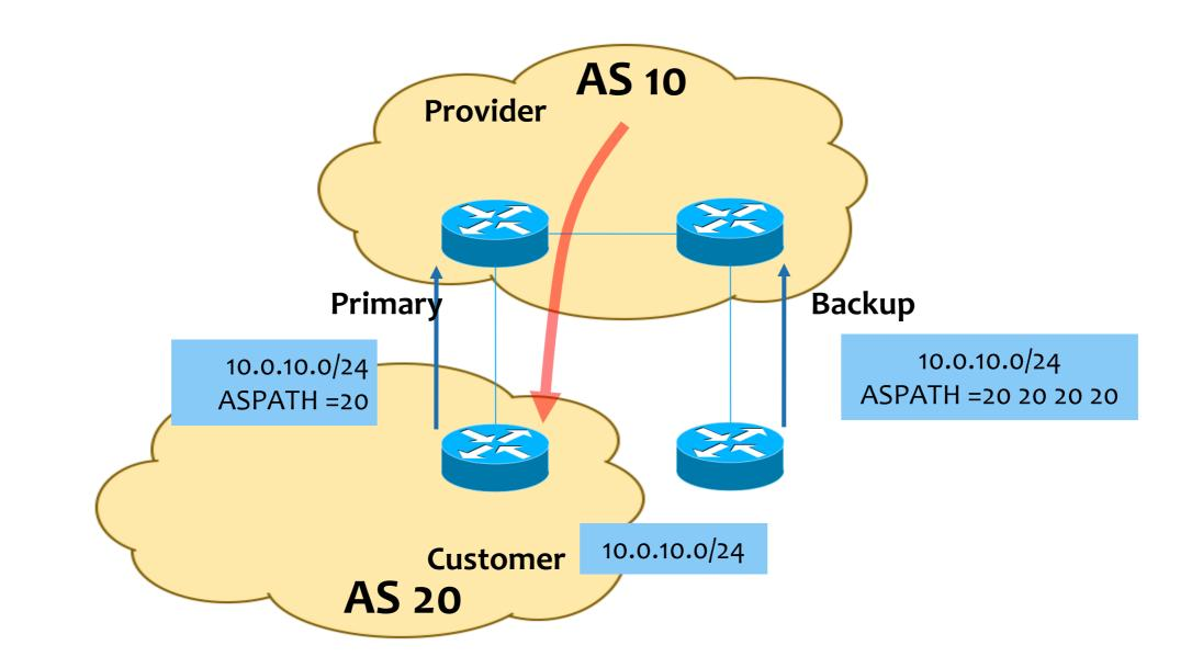
Prepending will (usually) force inbound traffic from AS 10 to take primary link  Customer purchased a new link from the second service provider which uses AS number 30 and decommissioned one of it's link from the old service provider
