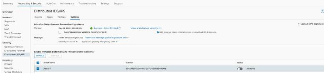
Figure 7.4 – Enabling distributed IDS/IPS on a cluster level
