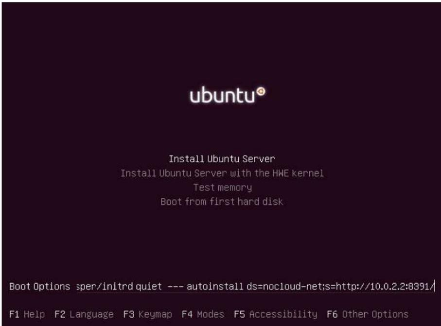
**Figure 13-9.** *Launching the automated installation*
