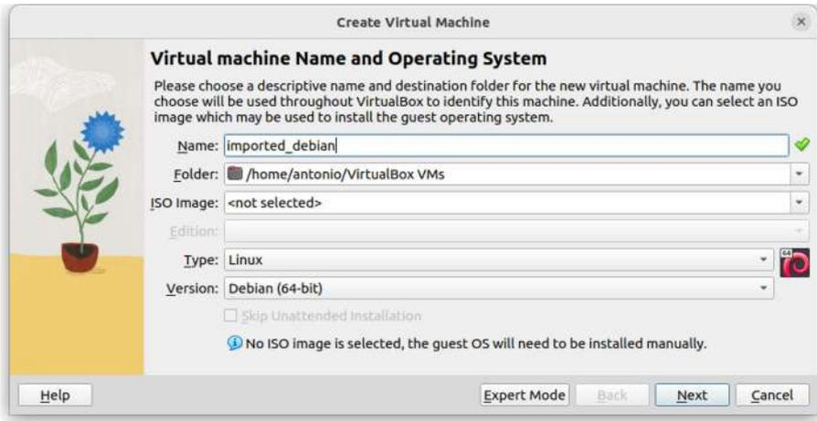
**Figure 5-3.** *Creating a new virtual machine in VirtualBox*
