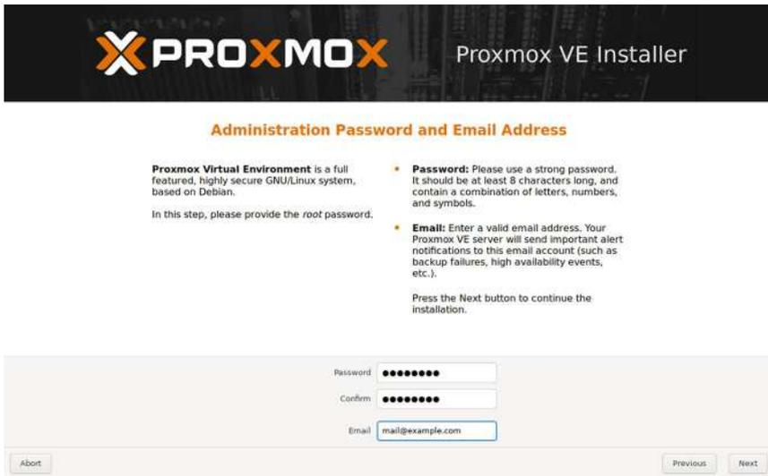
Figure 6-5. Installing Proxmox. Setting the root password
