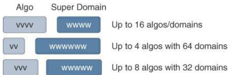
**Figure 3-53** SRv6 SID Block Carving (Large-Scale Deployment)
