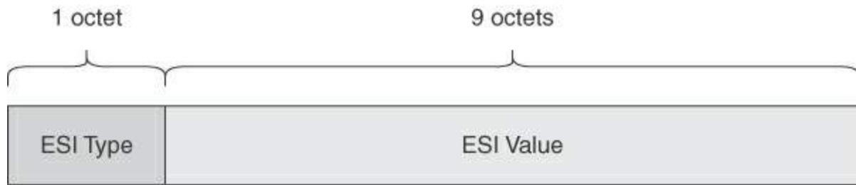
**Figure 6-11** *EVPN Ethernet Segment Identifier Format*
