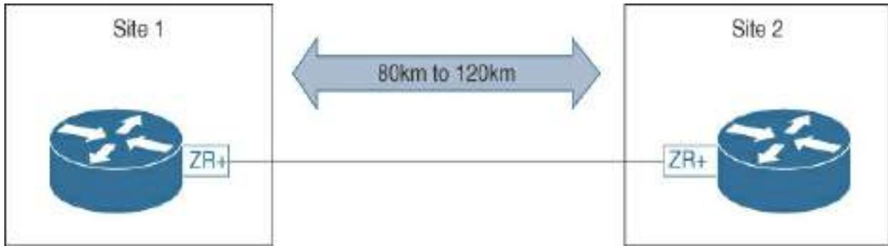
**Figure 10-8** *Simplified Long-Distance Connection*
