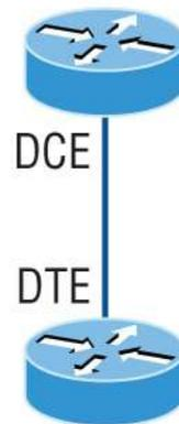
DCE side determined by the cable.
