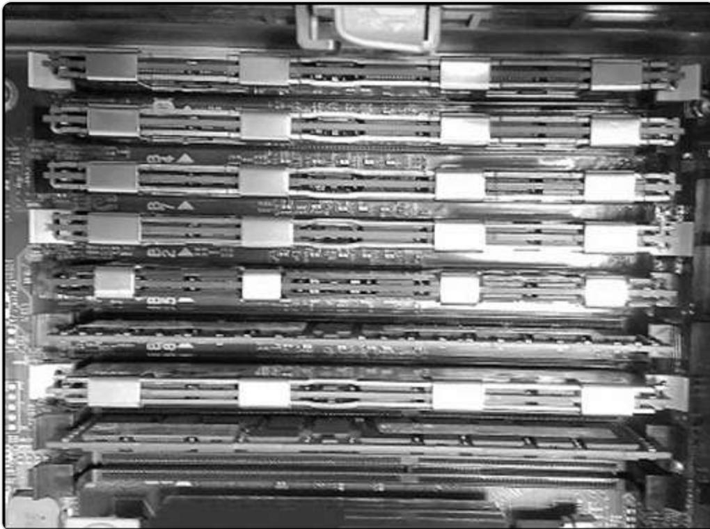
Figure 13.2 – ECC RAM modules placed in memory banks
