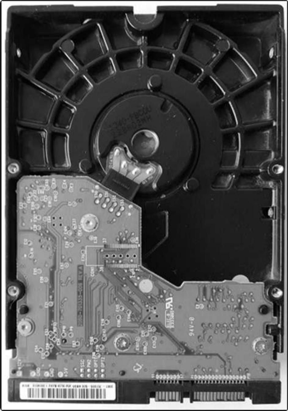
Figure 8.6 – Disk controller in an HDD
