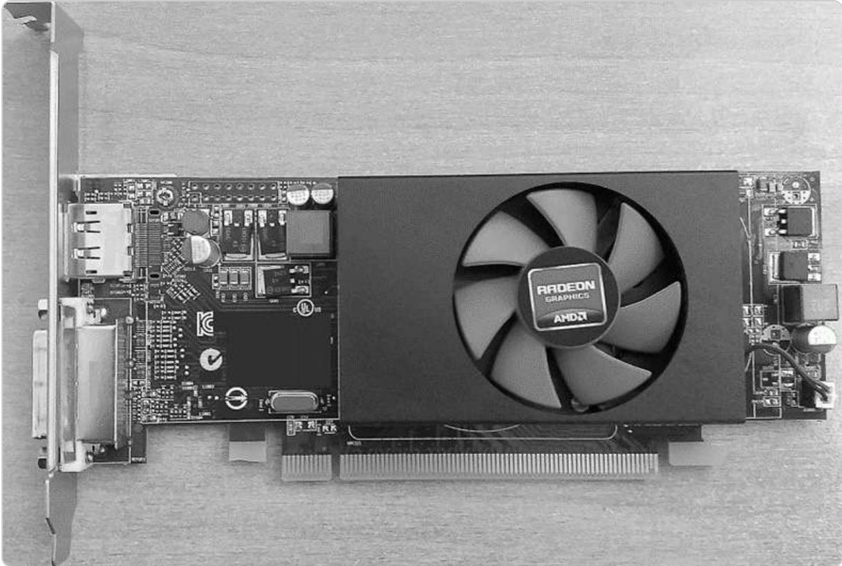
Figure 13.6 – AMD’s Radeon video graphic adapter
