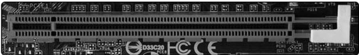
Figure 8.2 – The PCIe slot
