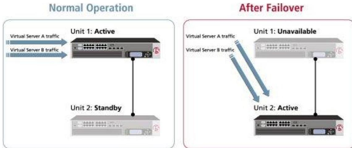
As you can see in the figure, unit 1 is in an active state, and unit 2 is in a standby state. With this configuration, failover causes the following to occur:
