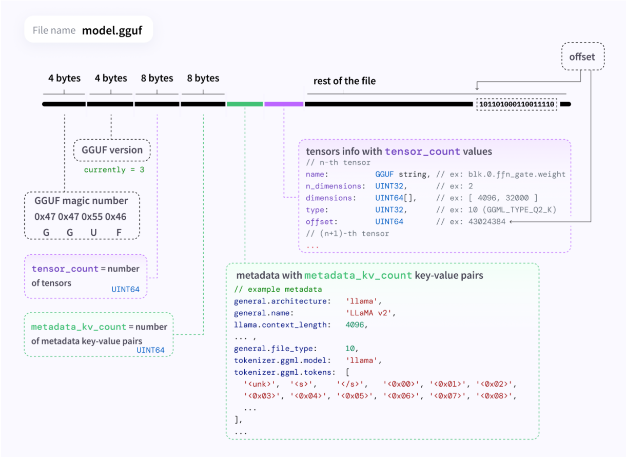
Figure 3-4. Internal structure of a GGUF file.
