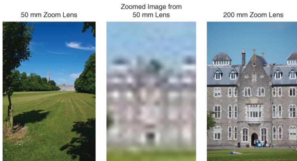
Figure 4-9 50 mm Zoom Lens versus 200 mm Zoom Lens
