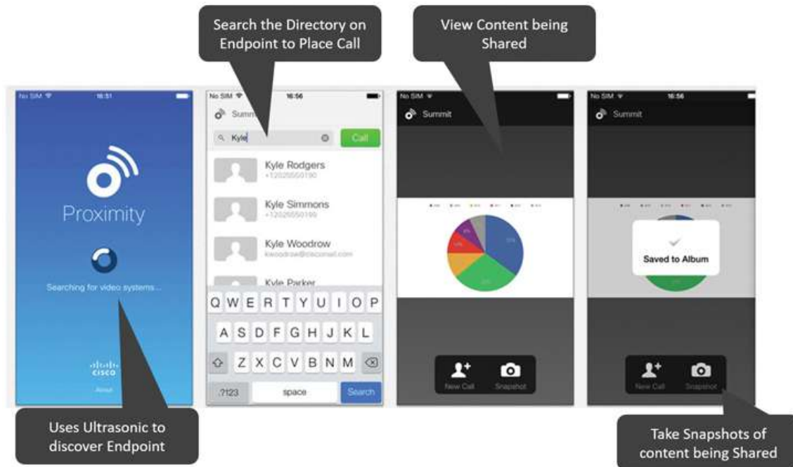
Figure 8-2 Intelligent Proximity for Content Sharing on a Smartphone
