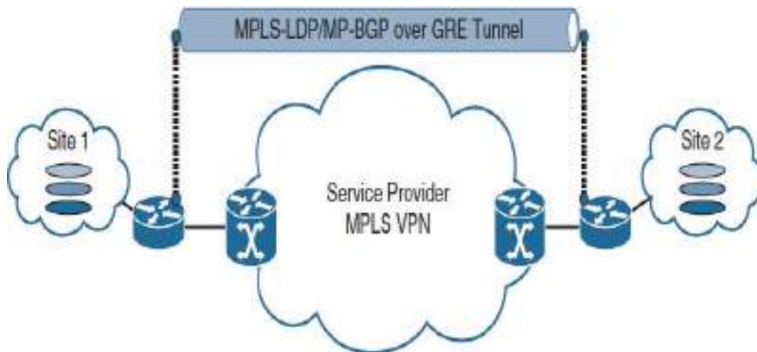
Figure 17-22 MPLS over Point-to-Point GRE Tunnel
