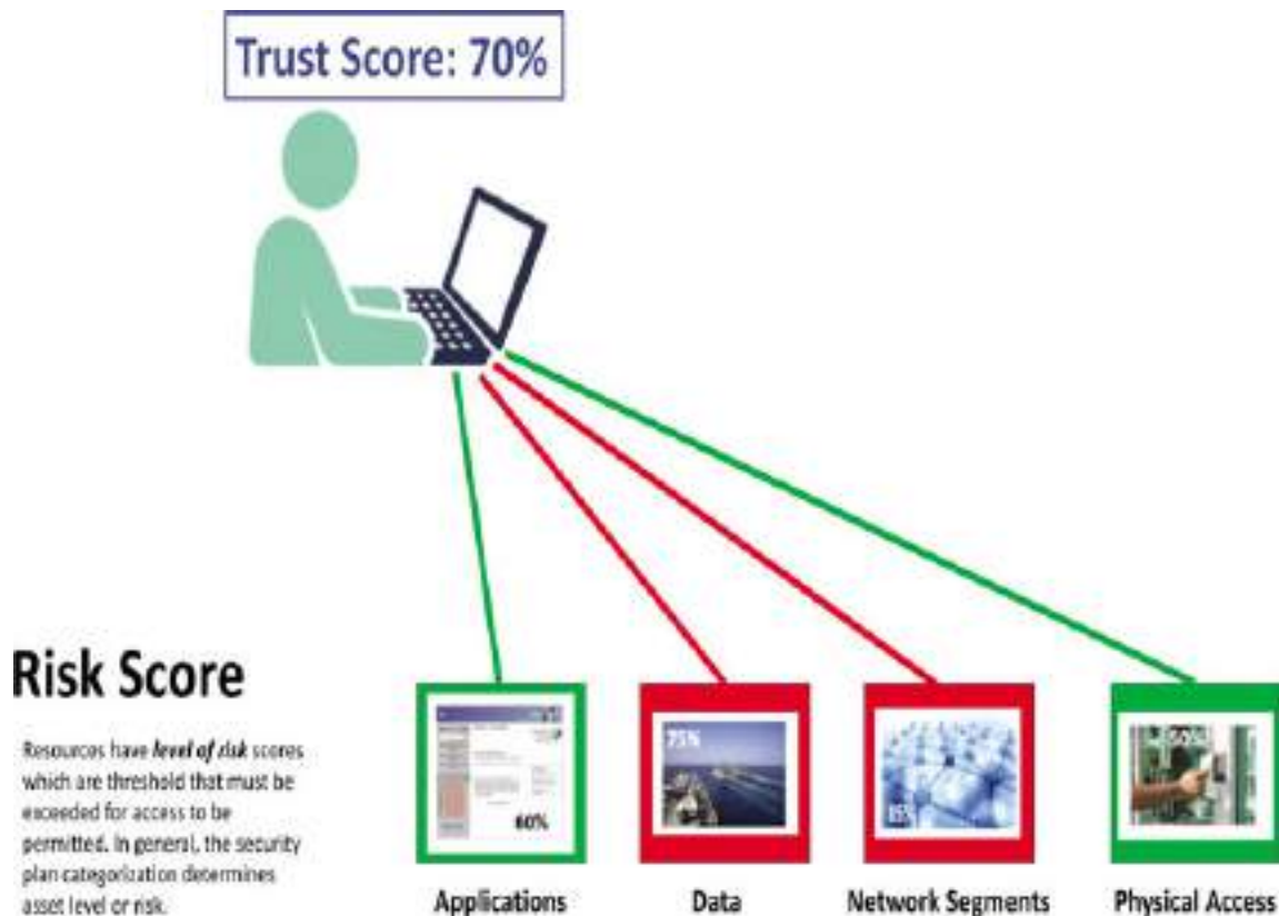
Figure 4-5 Zero Trust Architecture Concept of Trust Score vs. Risk Score
