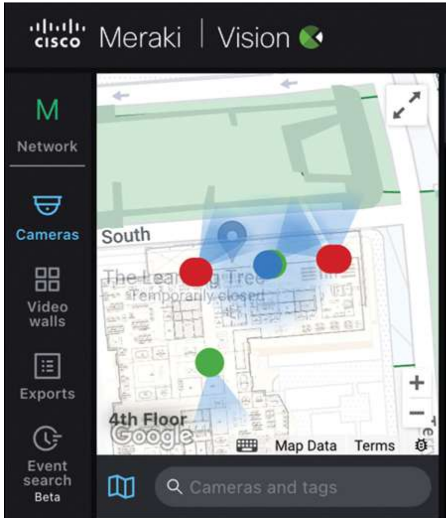
Figure 9-10 Relative Camera Positions on a Floorplan as Shown from the Meraki Vision Portal
