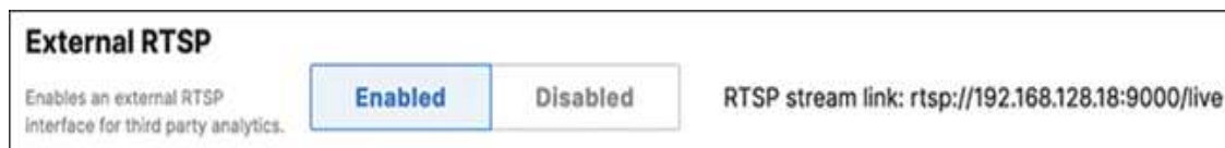
Figure 9-26 Enabling External RTSP
