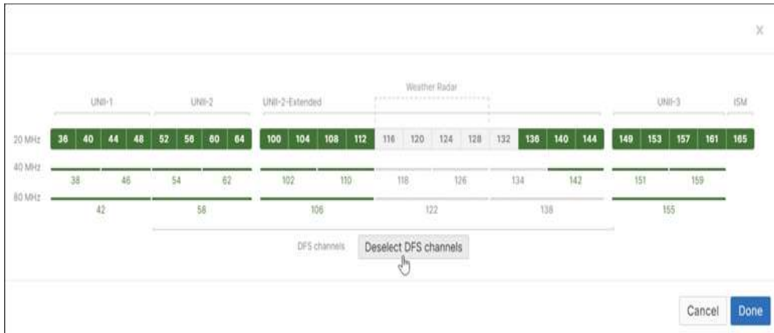
Figure 8-12 5-GHz Channel Availability Configuration with Non-Weather Radar DFS Channels Enabled
