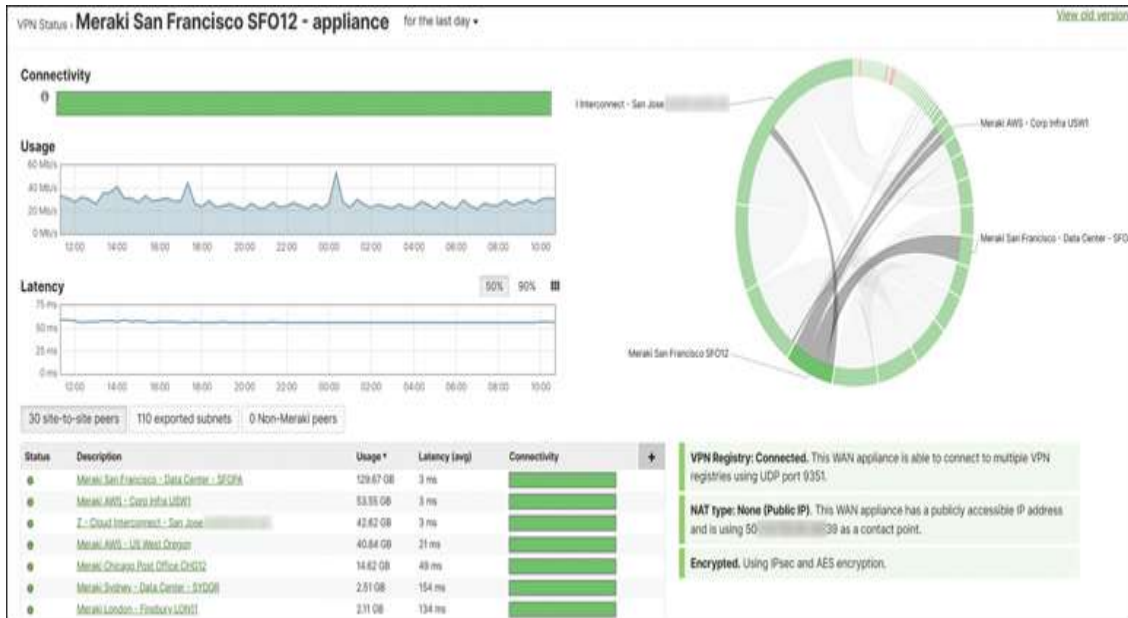
Figure 5-23 Network-level VPN Status Showing the Per-Peer Tunnel Data and Connection Details for the Device in This Network
