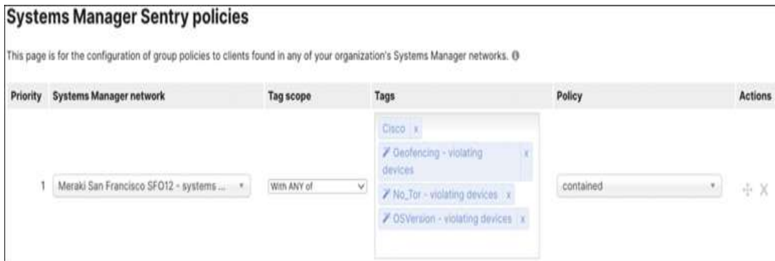
Figure 7-28 Sentry Policy Mapping Between SM Tags and Group Policies in the Dashboard
