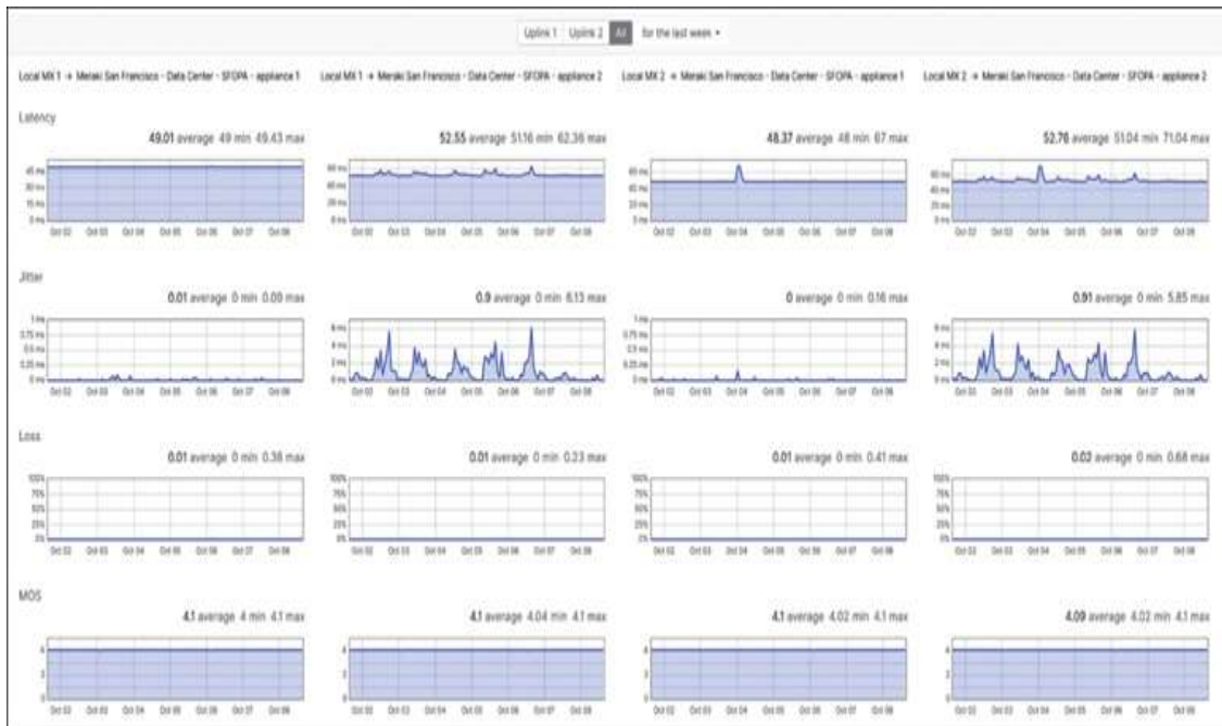
Figure 5-25 Per-Uplink VPN Monitoring Data Showing Historical Results for the Tunnels Between Each Uplink of Two Peers
