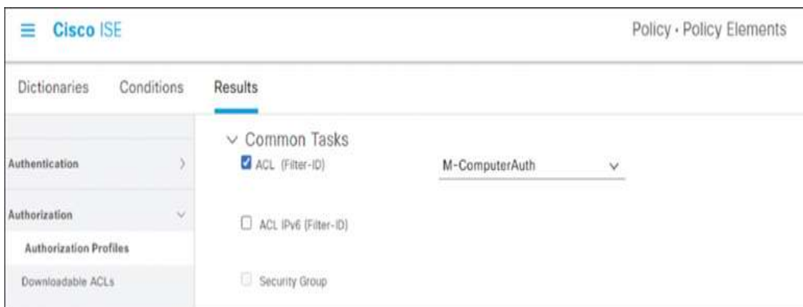
Figure 7-26 Mapping an ISE Filter-ID to a Corresponding Meraki Group Policy
