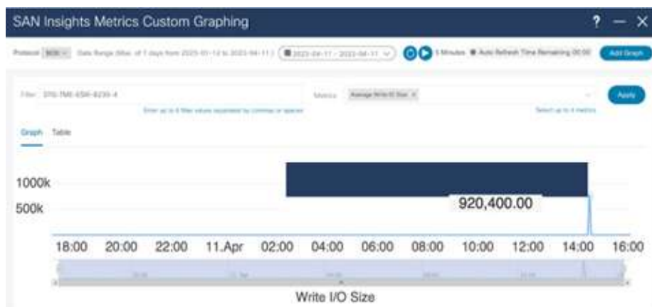
Figure 5-16 Write I/O size spike as shown in NDFC/DCNM SAN Insights
