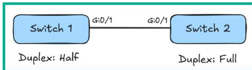
Figure 3.22: Duplex mismatch between switches
