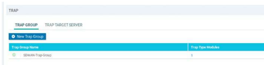
Figure 13-14. The finished trap group
