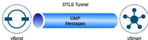
Figure 4-2. DTLS tunnel carrying OMP messages
