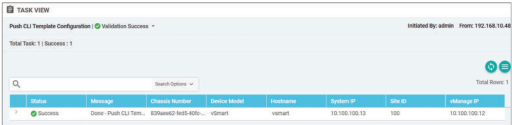
Figure 5-14: Changing vSmart to the vManaged Mode – Verification: Success.
