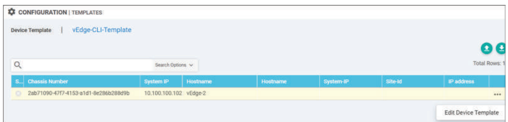
Figure 6-45: Attach CLI Template to vEdge – Edit Device Template#1.
