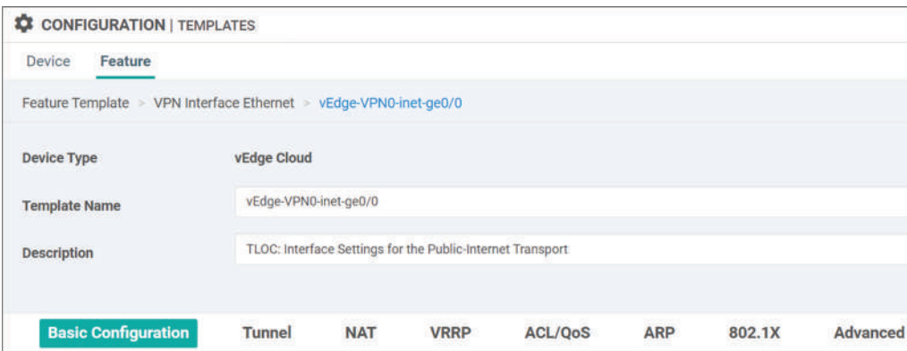
Figure 6-10: Feature Template – VPN: VPN Interface – Interface Basic Settings.
